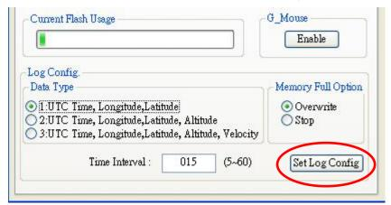
When you done the configuration setup, press the "**Set Log Config.**" button to save the setting to the receiver.
